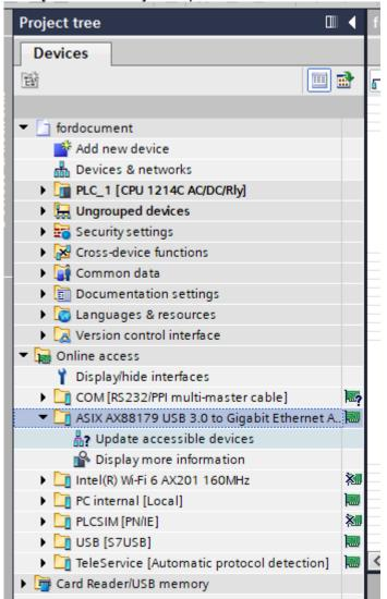
2 Double-click [Update accessible devices] to detect connected PROFINET devices
