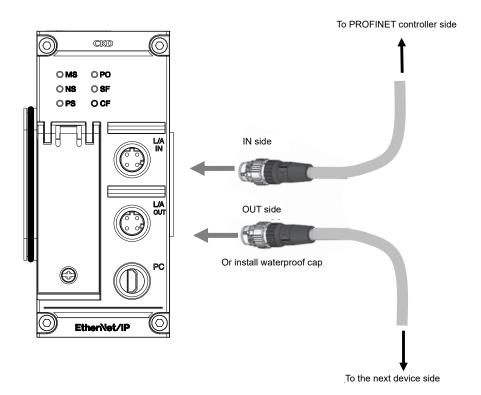
For PROFINET communication wiring, purchase a cable or connector that meets the following specifications:
