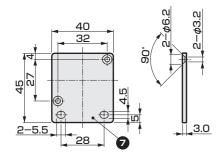
\* For mounting bracket Two flat head machine screws included
