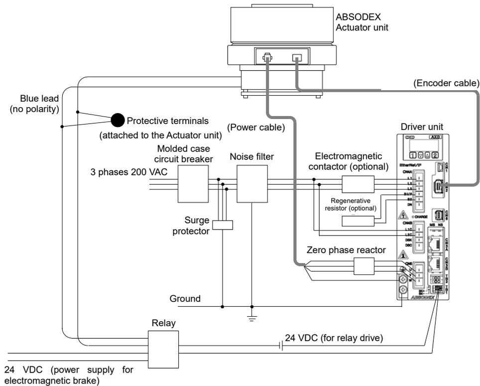
The strip length of wires must be 9 to 10 mm.
