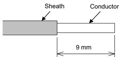
Stranded cable: Peel off the sheath of the cable and twist it to use.
