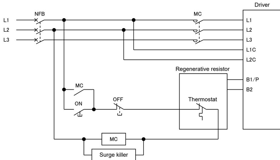
Refer to the figure below for wiring the regenerative resistor.
