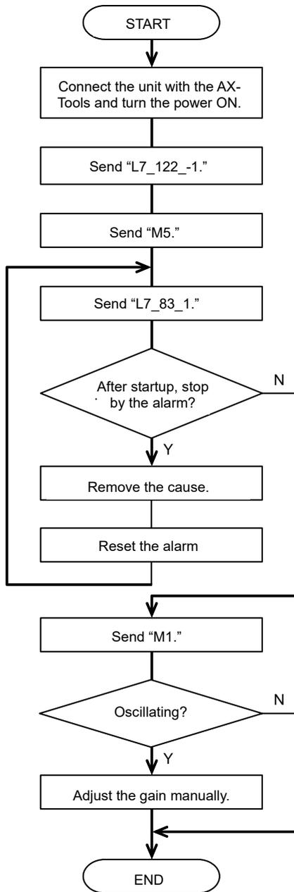
At the terminal mode of the AX-Tools, enter commands necessary for auto tuning.
