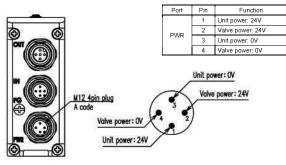
nded M12 connector (socket): loose wire type power cable Mfd by Omron Corporation XS2F-D421-080-0 Straight type
