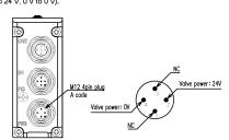
mmended M12 connector (socket): loose wire type power cable XS2F-D421-□8□-□ M12 power cable Straight type Note: □ differs depending on the cable specifications. Mfd by Omron Corporation
