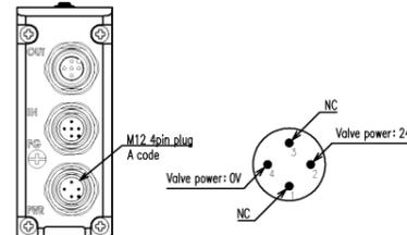
Recommended M12 connector (socket): loose wire type power cable
