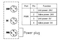
Recommended M12 connector (socket): loose wire type power cable XS2F-D421-□8□-□ Straight type Mfd by Omron Corporation
