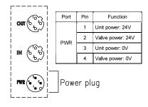
ended M12 connector (socket): loose wire type power cable
