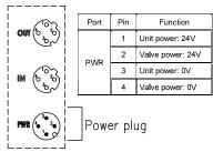
Recommended M12 connector (socket): loose wire type power cable XS2F-D421-⊓8⊓-□ Straight type Mfd by Omron Corporation
