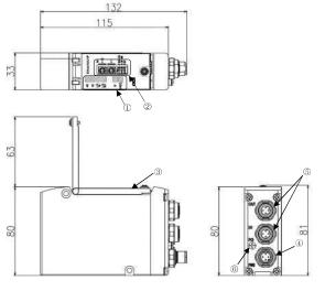
① LED Indicate the status of the device and network with MS, NS, L/A IN, L/A OUT, ST and PW(V).
