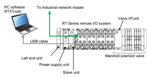
Two or more manifold solenoid valves can be connected, up to a maximum of 24.
