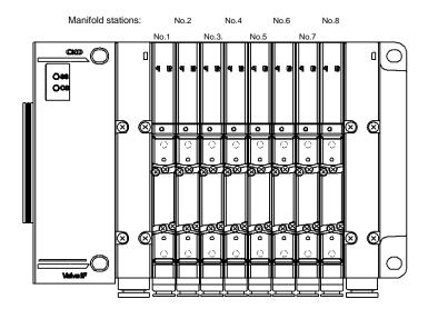
As an example, the diagram on the left (shows) a double solenoid type solenoid valve equipped in 8 stations.
