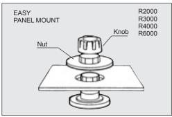
Note: Before mounting a knob, a nut should be set. (For R2000, the nut can be detached alone without dismounting the knob.)
