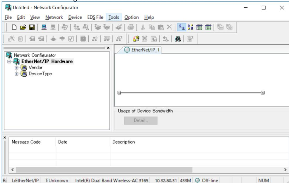
Select [Tools] - [Setup TCP/IP Configuration]. (In the example, the new IP address is set to 10.17.34.1)
