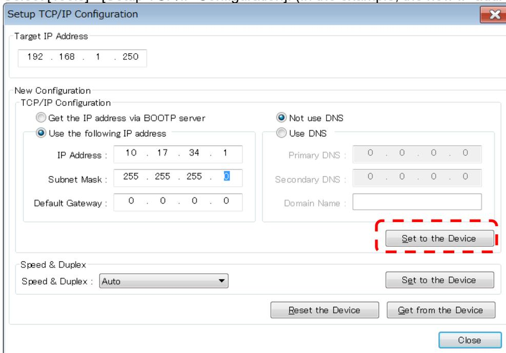
Press "Set to the device" and write the new IP address.
