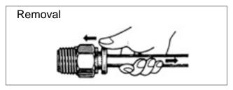
While pressing down on the push ring with your fingers, the tube can be removed by pulling on it.
