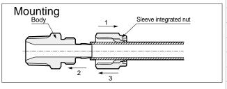
Pass tube through the sleeve integrated with the nut. Insert tube into the main body, and tighten the sleeve integrated with the nut until it contacts the body.
