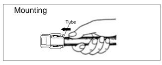
Push the tube in until it contacts the tube end. Check that the tube does not come off the fitting. Tube inserts 15 to 21 mm from the end of the fitting body. The end of the mounted tube must be cut at a right angle.
