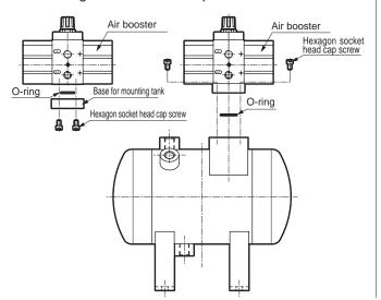
■ Installation of an air tank and regulator after the air booster is recommended for attaining stable secondary pressure.
