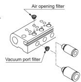
■ If the foreign matter trapping capacity of vacuum suction is insufficient for your application, you can either use the optional insert vacuum filter or install vacuum filters in between the pad/nozzle and valve.
