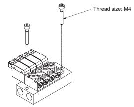
Tightening torque: 0.6 to 0.8 N⋅m
