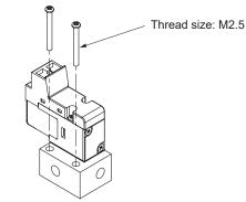
Tightening torque: 0.20 to 0.25 N⋅m
