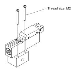
Tightening torque: 0.15 to 0.2 N⋅m
