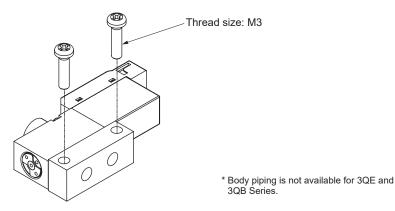
Tightening torque: 0.25 to 0.4 N·m
