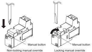
Do not operate with excessive force. The solenoid valve could be damaged.
