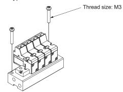
Tightening torque: 0.25 to 0.4 N⋅m
