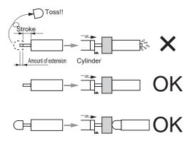
■ A guide is required if the colliding object vibrates. Install a secure guide on the colliding object if the colliding object vibrates or if force is applied to the piston rod at an axial right angle direction. ■ When there is the risk of static electricity building up in an explosive environment
