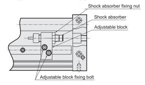
Full stroke adjustment volume (adjustment volume per full stroke adjustable bracket)
