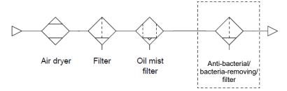
Make sure that substances such as chlorine do not become mixed with the compressed air when using a water lubricated type compressor circuit.
