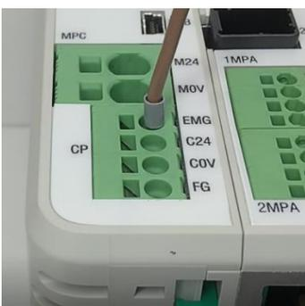
Make sure the wire is locked and does not come off.
