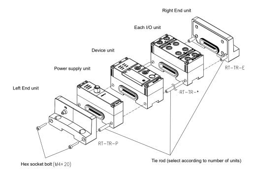
Connect the following tie rods in advance. Select as few tie rods as possible.
