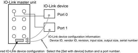
Registered IO-Link device configuration Select the [Set with device] button and a port number. information
