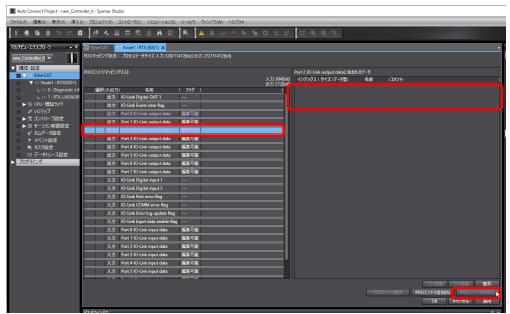
Delete the default PDO entries "Port 2 byte 0 output data" to "Port 2 byte 3 output data".
