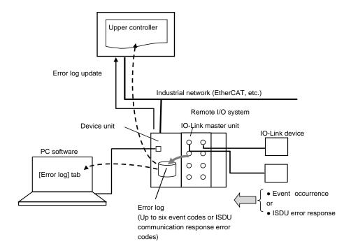
Up to six event codes or ISDU communication response error codes are stored in the device unit as an error log. They can be read using one of the following methods:
