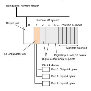
In this example, the size of the process input on port 2 is 8 bytes. So the size of the communication unit (e.g., PDO for EtherCAT) must be changed from the default 4 bytes to 8 bytes on the configuration tool of the upper controller.
