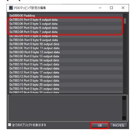
For example, if the output size of the IO-Link device on port 0 is 8 bytes for the PDO "Port 0 IO-Link output data" per module, perform edits as follows:
