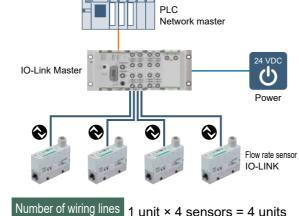
General analog input units do not supply power to the sensor.
