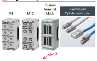
Input the digital signal (ON/OFF signal). Signals from the 2-wire/3-wire cylinder switches are fetched and fed back to the PLC through the device unit of the remote I/O. This enables network management. Using a Y-splitter connector, two switches can be input through a single port. (M12 type only)
