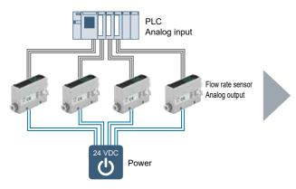
Number of wiring lines 5 units × 4 sensors = 20 units
