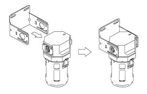
Slide C shape bracket sideway making its projected rail matching with the grooved rail on the unit.
