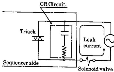
Regulate the residual leaking current within the following limitations;
