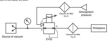
Do not expect the pressure on the secondary side to remain for a long period. Take measures to remove residual pressure as necessary.
