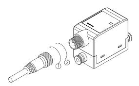
When screwing in the connector, screw in the lollet part instead of the cable body.
