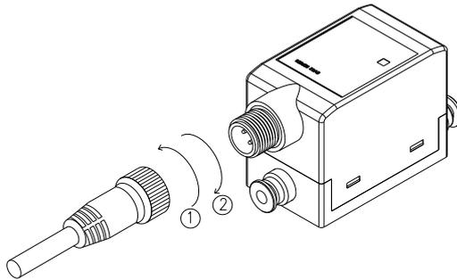
**When screwing in the connector, screw in the knurled part instead of the cable body.**
