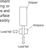
to the fingers, consider the impact to the gripper body and tighten it with a wrench so that the fingers are not twisted.
