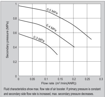
Note) Air booster needs approx, twice secondary side flow rate (max.) for primary side due to structure. Confirm that the instantaneous flow rate is within the curve
