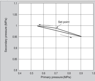
Pressure characteristics show variation of set secondary pressure according to primary pressure variation.
