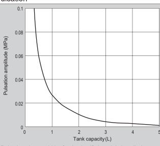
Pulsation shows width of pulsation if air tank is installed onto secondary side of air booster.
