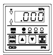
[000] turns ON. Zero point adjustment is finished
