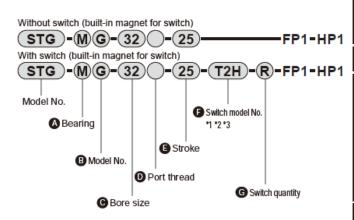
Description Code A Bearing Metal bush bearing Ball bearing В B Model No. Rubber scraper Bore size (mm) 12 ø16 20 ø20 25 32 ø25 ø32 40 ø40 50 ø50 63 ø63 80 ø80 100 ø100 Port thread Blank M5 (ø12 to ø16) Rc thread (ø20 to ø100) NPT thread (ø20 and over) (made to order) GN G thread (ø20 and over) (made-to-order product) (B) Stroke (mm)
