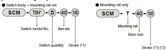
Note 1: Indicate X if the stroke length exceeds 300 mm. If exceeding 300 mm, a short rail (with 100mm switch adjustment travel distance) will be included per switch.
