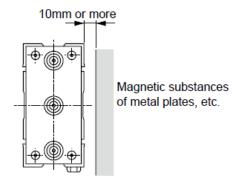
• The cylinder switch may malfunction if the cylinder units are placed adjacently. Make sure to provide the following distance between each unit.
