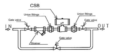
Use union fittings or flange fittings and provide a bypass pipe to facilitate maintenance.
