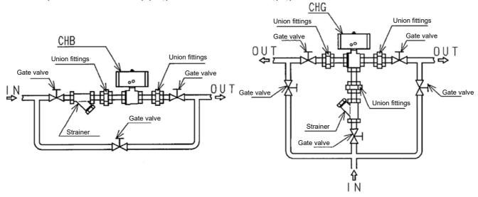
Use union fittings or flange fittings and provide a bypass pipe to facilitate maintenance.
