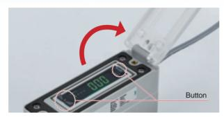
With the LCD display, button operation is possible by opening the cover.
