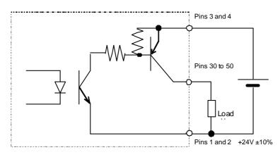
Rated voltage: 24V ±10% (including ripple) Rated maximum current: 30mA (Max.)
