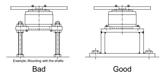
2) When ABSODEX can not be directly mounted on a machine, it should be mounted on the deck of high rigidity.
