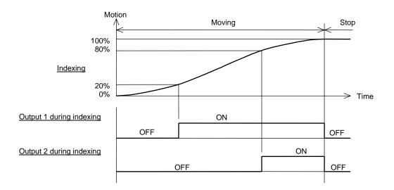
Fig. 5.20 Example of Output During Indexing (In case of PRM33 = 20, PRM34 = 80)
