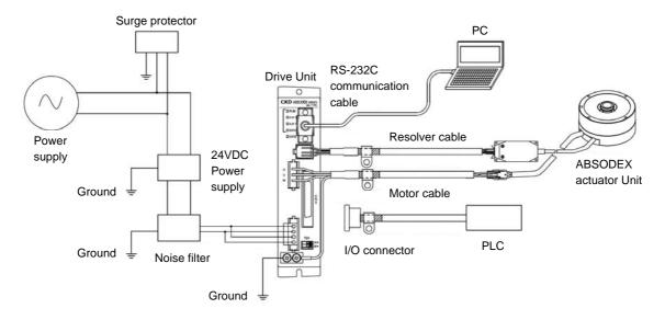
Fig. 3.1 System Configuration
