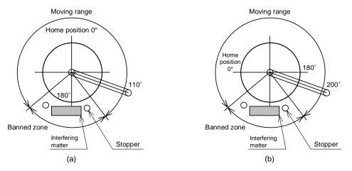
Fig. 8.6 Coordinate System Setting
