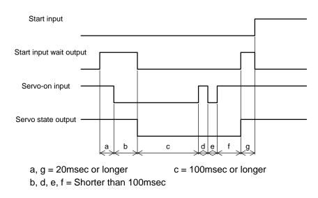
Fig. 5.13 Timing Chart of Servo-on Input
