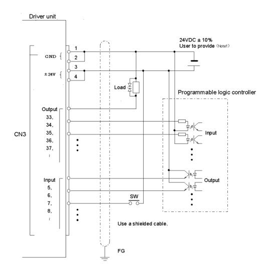
(Note1) The wiring is opposite from AX9000MU with NPN specification.
