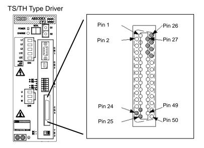
Fig. 5.2 CN3 Connector (TS/TH Type Driver)
