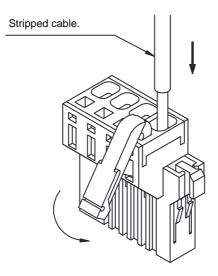
Fig. 3.4 Cable Insertion Method
