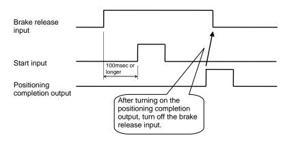
Fig. 5.12 Timing of Brake Release Input
