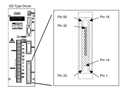
Fig. 5.1 CN3 Connector (GS Type Driver)
