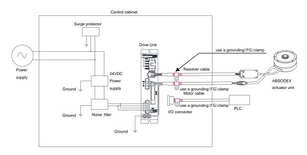
Fig. 15.1 Installation of Driver (in case of 3 phases)
