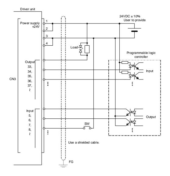
Fig. 3.5 Connection Example NPN specification
