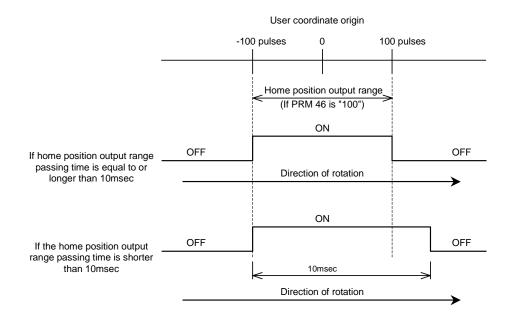
Fig. 5.21 Home Position Output Timing
