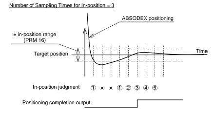
Fig. 7.6 Position Completion Output
