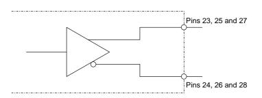
Output type: Line driver Line driver to be used: DS26C31 Recommended line receiver: DS26C32 or equivalent
