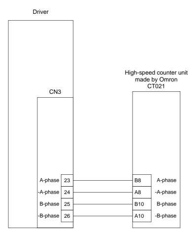
Fig. 3.14 Wiring Example of System Operating with Encoder Outputs
