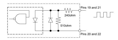
Rated voltage: 5V ±10% Max. input frequency Line driver: 1Mpps Open collector: 250Kpps
