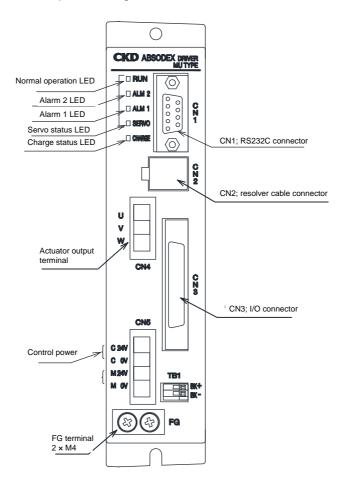
Fig. 3.2 MU Type Driver Panel
