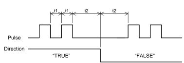
Fig. 5.23 Pulse & Direction Inputs
