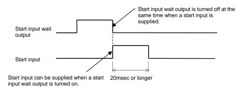
Fig. 5.11 Start Input Timing
