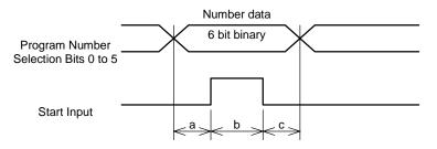
a = 10msec or longer b = 20msec or longer c = 0msec or longer Fig. 5.10 Program Number Setting Timing
