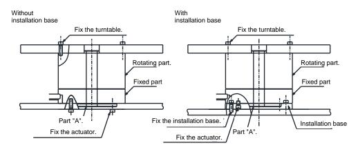
Fig. 2.1 Actuator Installation
