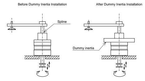
Fig. 2.5 Dummy Inertia Installation 3
