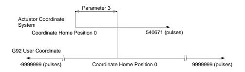
Fig. 6.1 ABSODEX Coordinate System
