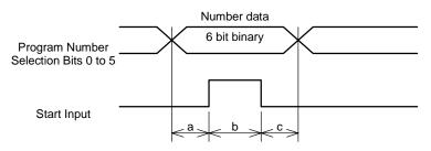
a = 10msec or longer b = 20msec or longer c = 0msec or longer Fig. 5.9 Program Number Setting Timing
