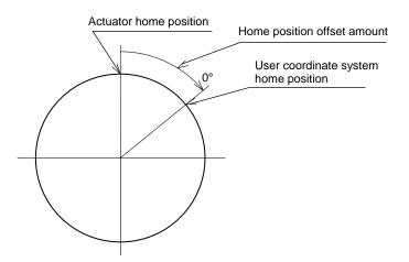
Fig. 7.2 Amount of Home Position Offset & Coordinate System Home Position
