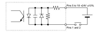
Rated voltage: 24V ±10% (including ripple) Rated current: 4mA (at 24VDC)
