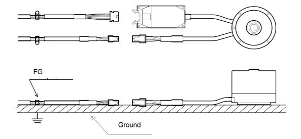
Fig.15.2 Grounding Example on Actuator Side
