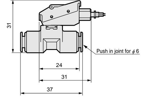
Sensor separate type (stainless steel diaphragm sensor)
