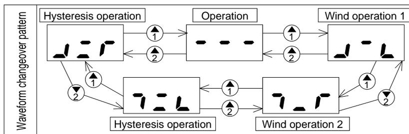
Note 1. When using for a window operation, provide an interval of 3%F.S. or more between the 2 set values.
