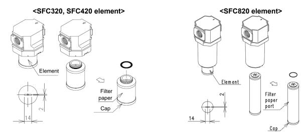
If the element is hard to turn by hand, insert a flat blade screwdriver into the slit in the cap at the bottom of the element and use it to turn the element.
