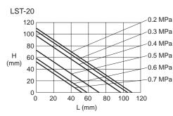
When LST-20 is selected, the intersecting point of L: 40mm and H: 20mm will be inside the supply pressure line of 0.5MPa, and so it can be used.
