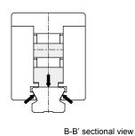
When air is discharged from the lock release port, the piston and the tapered movable swash plate connected to the piston are moved in the direction of the arrow by the spring lock. The amplifying effect of the taper is passed through roller B so that the lock shoe presses the rail with force.
