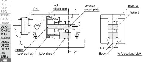
When the lock release port is pressurized with air, the piston and the tapered movable swash plate connected to the piston move in the direction of the arrow, releasing the contact of roller B and the movable swash plate.
