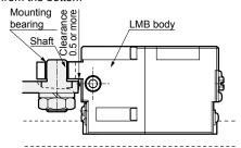
Insert a shaft (pin) into the bearing for installation and connect with the slide table. At this time, provide clearance as shown in the figure above. (Due to the structure, the LMB body lowers during locking, so if the bearings are fixed without a clearance, the lock will not be applied.)
