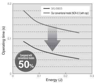
\* Data are reference values at cylinder thrust 60 N, room temperature. Operating time varies according to collision conditions.
