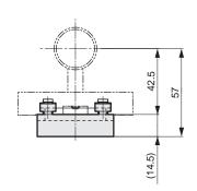
Fitting/high load (RJ-H)
