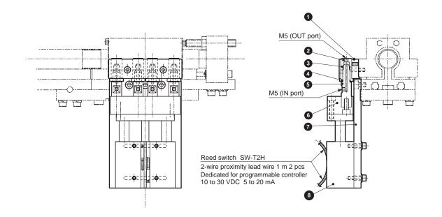
Air supply unit/high load (PR-H)
