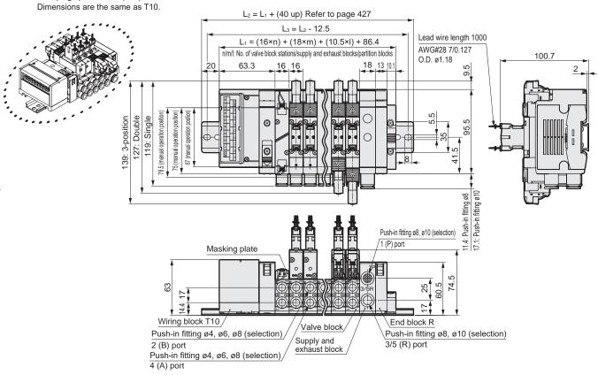
Common terminal block (M3 thread) right side (T10R) Note: Clamping specification (T11R) is also available.
