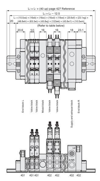
This diagram is one example of the many free combinations available for the mix manifold. With the dimensions listed below, configure combinations with reference to the previous page.
