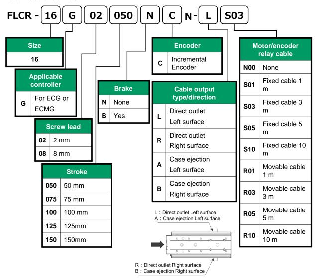
If you select other than "N00" for "Motor/encoder relay cable", a motor/encoder relay cable is included as an accessory.
