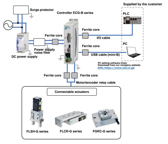
The above diagram is a configuration diagram for the parallel I/O specification. For other interface specifications, refer to the instruction manual for each interface specification.
