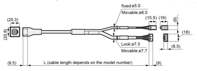
The actuators shipped on or before September 2022 include the relay cable of which model number is "EA-CBLME2-□□". Refer to "7.2 Cable specifications" for details.
