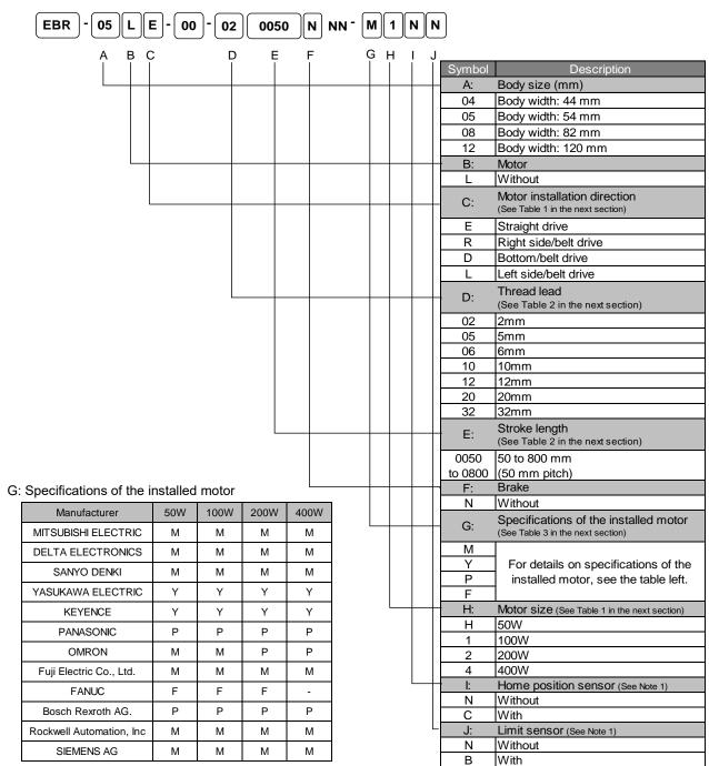
Note 1) The home position sensor and limit sensors are used together.
