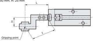
When LSH-A20D is selected, the intersection of L:50mm and  $\rm H:25mm$  will be inside the supply pressure line of 0.5MPa, so it can be used.
