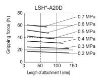
For example, when supply pressure is 0.5 MPa and attachment length is 50 mm, the gripping force is 40 N.
