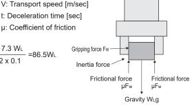
Note) Allowance is required for transport coefficient K due to impacts during transportation, etc. Even when the coefficient of friction  $\mu$  is higher than  $\mu$  = 0.1, set transport coefficient K from 10 to 20 or more for safety.
