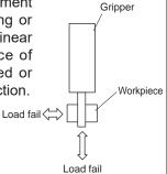
Attachment mounting method When mounting the attachment to the fingers, consider the impact to the gripper body and tighten it with a wrench so that the fingers are not twisted.
