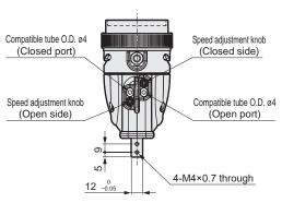
Dimensions when attachment is installed
