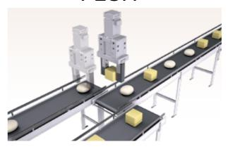
Gently grasp various workpieces that are easy to deform, and with just one actuator.
