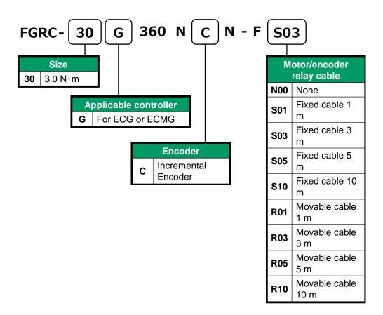
If you select other than "N00" for "Motor/encoder relay cable," a motor/encoder relay cable is included as an accessory.
