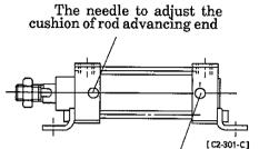
The needle to adjust the cushion of rod retracting end
