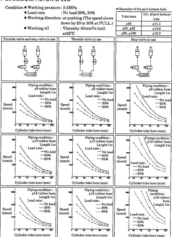
Note: The speed of hydraulic cylinder differs depending or the kind of valve such as throttle valve or stop valve, and the size of lower hole on piping port for the cylinder.
